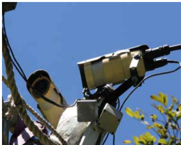
Figure 4.2.8 Camera and sensors used to monitor use of canopy bridges at Palmerston Highway (Cohen 2008).
