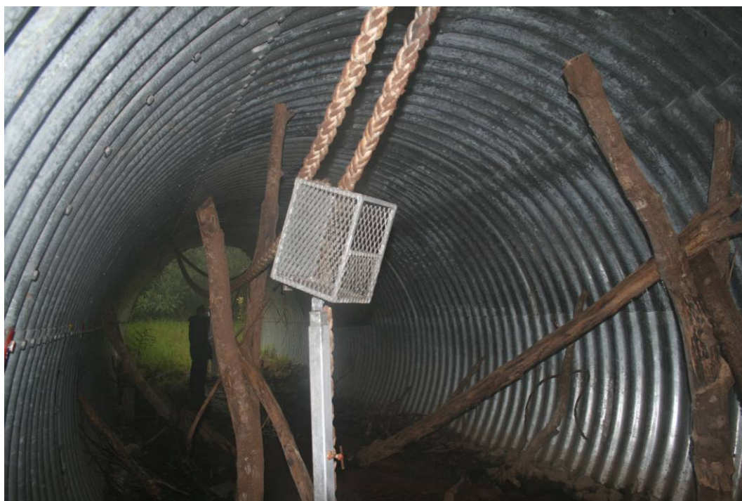
Figure 4.2.9 Vandalism resistant cage for still camera in fauna underpass, East Evelyn (Scott 2007).
